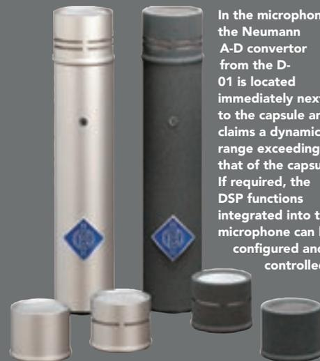
In the microphone, the Neumann A-D converter from the D-01 is located immediately next to the capsule and claims a dynamic range exceeding that of the capsule. If required, the DSP functions integrated into the microphone can be configured and controlled
