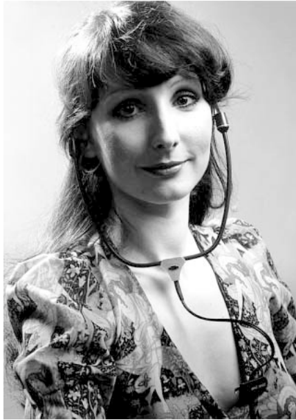
Fig. 32 Real-head stereo microphone (MKE 2002, Sennheiser)
